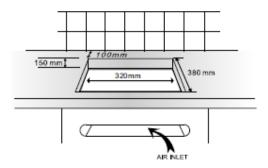
• In the front of cabinet, under the location of the ceramic hob, open an air inlet of more than 100cm<sup>2</sup> as shown below. If the cabinet is not sealed, then an air inlet is not necessary as it is just for heat elimination purpose.
